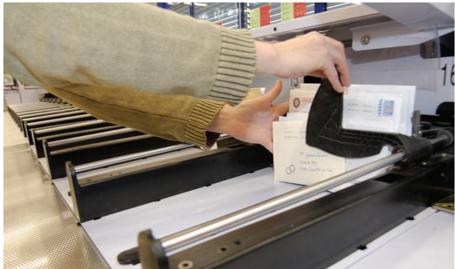
MARS can process up to 40,000 mailpieces per hour
