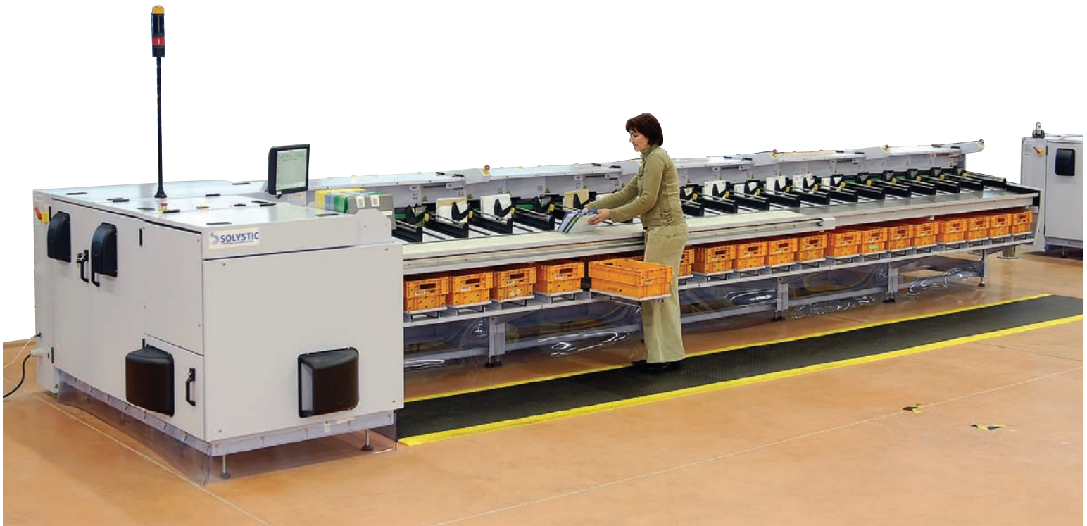
The compact and ergonomic design of the SOLYSTIC MARS mail sorting equipment means that it can fit into any branch office
