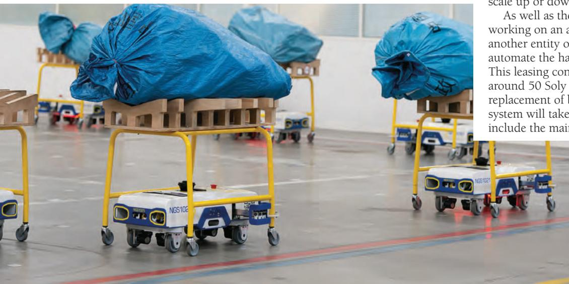
Soly Move has been designed to autonomously sort and transport baggage and irregular-shaped parcels in logistics operators' hubs
