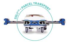
With Soly™, SOLYSTIC has created the first ever mobile robot able to prepare deliveries by sorting parcels according to the order of distribution.
